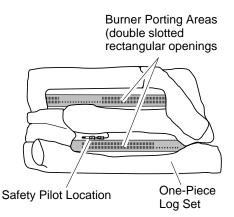
Figure 16 - Top View of One-Piece Log Set on Gas Log Heater
